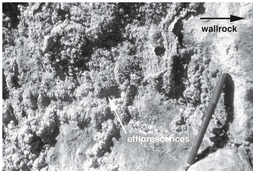
Fig. 2.7. Secondary gypsum efflorescences encrusting wallrock in the Mary Kathleen open pit, Australia. Field of view 50 cm
