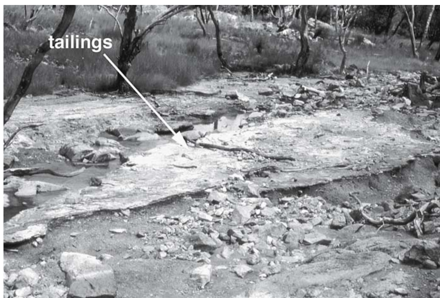
Fig. 4.7. Sulfidic tailings layer in ephemeral creek bed downstream from the derelict lead-zinc Webbs Consols mine, Australia. The tailings contain wt.% levels of arsenic, lead and zinc
